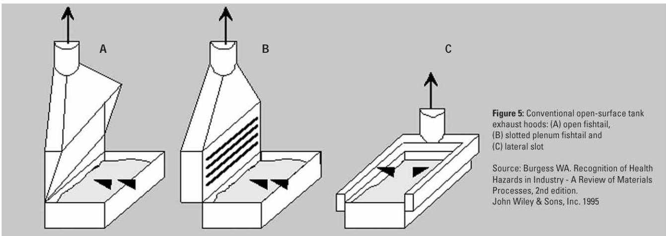
**Figure 5:** Conventional open-surface tank exhaust hoods: (A) open fishtail, (B) slotted plenum fishtail and (C) lateral slot
